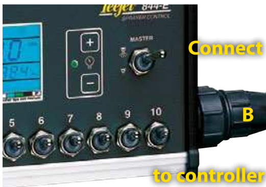
Figure 6: BoomPilot harness to flow control harness
